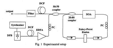
The total length of the cavity was 24.25 m corresponding to a fundamental frequency of 7.98 MHz. The external pulse train was generated from a 5 GHz gain switched DFB laser diode operating at 1548.5 nm. These pulses were compressed to 7.5 ps with a dispersion compensating fiber (DCF) and were amplified in an EDFA. For best performance, the polarization state of the external pulse train was adjusted with a polarization controller before insertion in the ring cavity.
